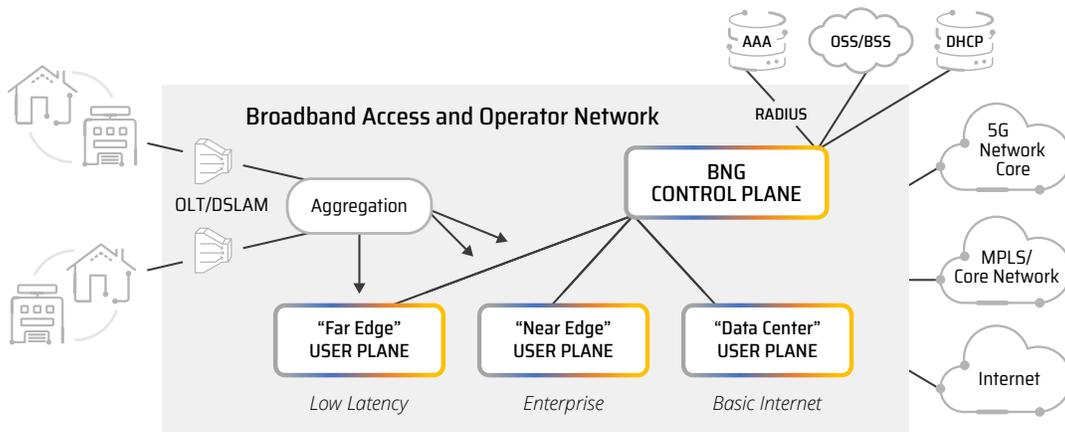
**FIGURE 2:** Benu Disaggregated Virtualized BNG (CUPS Architecture)
