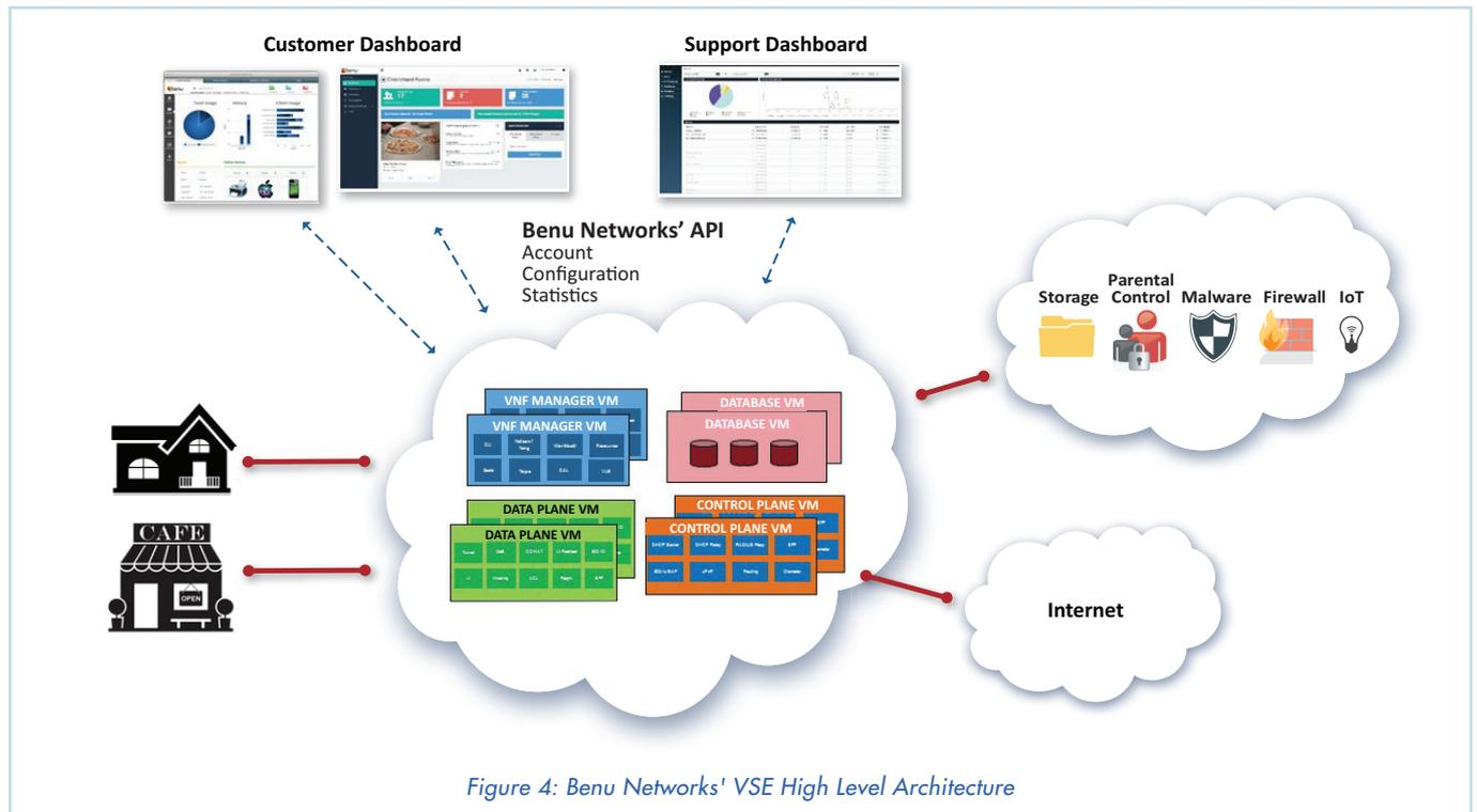
Figure 4: Benu Networks' VSE High Level Architecture
